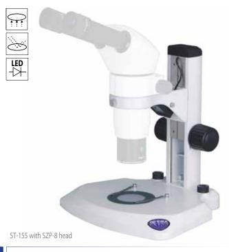
Modern, large plain stand equipped with **LED transmitted and incident illumination**, both with **intensity control**. It comes complete of head holder and focusing mechanism.
