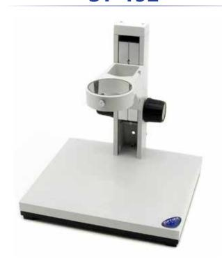
Large, simple plain stand with head holder and focusing mechanism. **Fixed arm type.**
