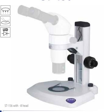
Modern, large plain stand equipped with **LED transmitted and incident illumination**, both with **intensity control**. It comes complete of head holder and **coaxial coarse and fine focusing system**. Base size: 330x285 mm. Height: 38 mm. Fixed arm height: 340 mm. Head not included.
