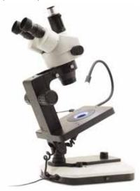
Vertical position for standard gem analysis with darkfield illumination and polarizing tecnique
