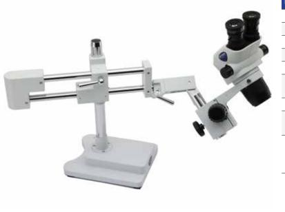
Binocular stereomicroscope with extremely stable, hinged and long overhanging stand complete of head holder and focusing system for observation of particularly large specimens. The head can be easily tilted for inspection at oblique angles ideal e.g. for stone setters. Smooth horizontal and vertical movement are ensured.
